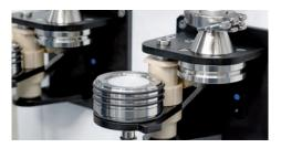
THE USER-FRIENDLY, lifting and tilting membrane holder includes three individual cascade rings with tweezer leads for safe and simple membrane fitting and removal of 0 47 mm membrane filters.
